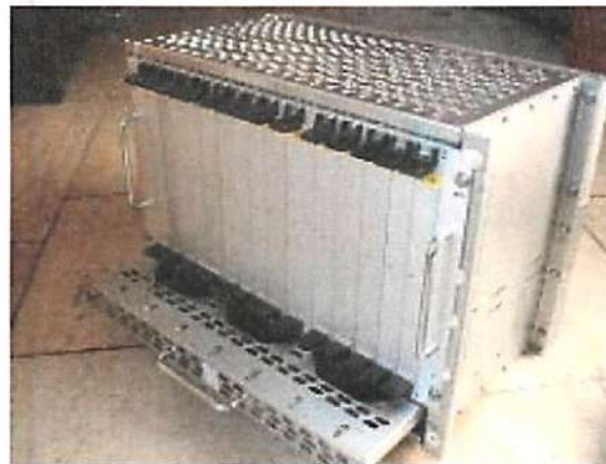
Figure 2 : WCR equipment with CMV and fan racks
